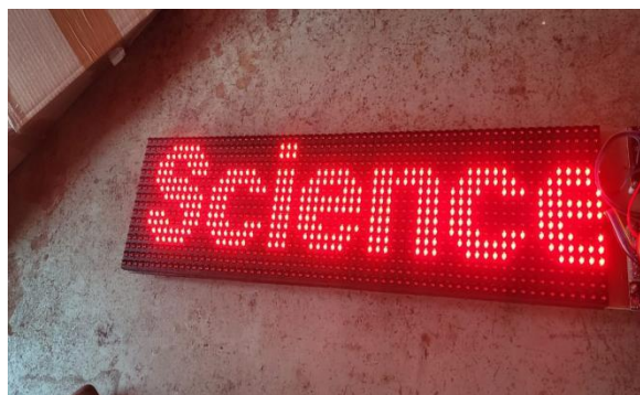
Fig9: showing the notice displayed in the LED display received from the Wi-Fi module
